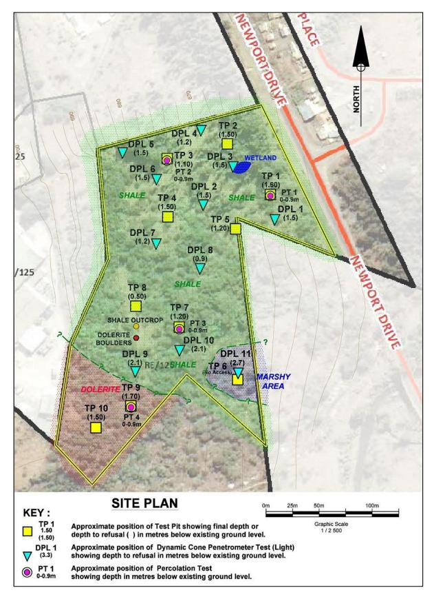
Figure 1: Site Plan showing layout of site and positions of Geotechnical Tests
