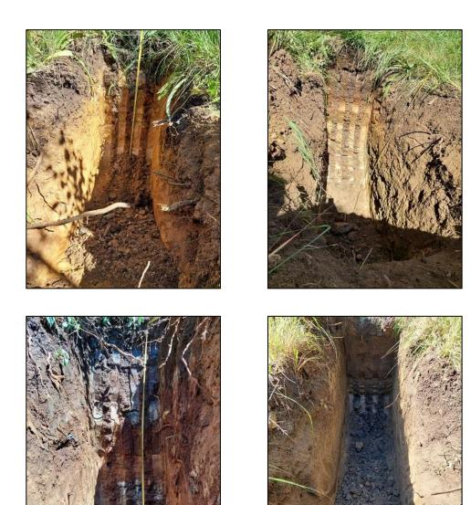
Plates 11 to 14: Typical soil profiles encountered beneath the site; clayey residual soils overlying the generally shallow, completely to highly weathered shale rock of the Pietermaritzburg Formation. The general dip and dip direction of the shale beds is 10 to 15° to the east.
